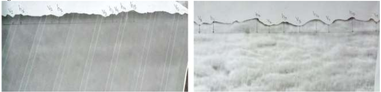
Avg. roughness: (a) 38 SWG with De-Ionised water (b) 38 SWG with 0.02 % Al 2 O 3
